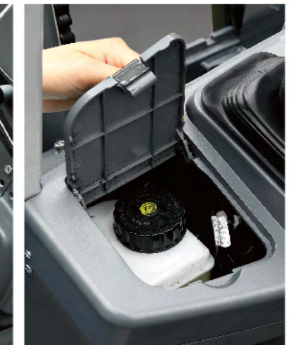
Brake fluid within reach, easy to check and refill
